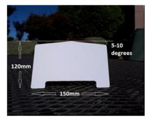
All individual elements rise to a 'peak' which runs the length of the element. The 'peak' rises at an angle of 5-10 degrees, meeting on the centre line of each element. All individual elements: height from ground at peak = 120mm. Depth = 150mm. Width = 1200mm. Subsequent elements may escalate in width to aid stacking.
